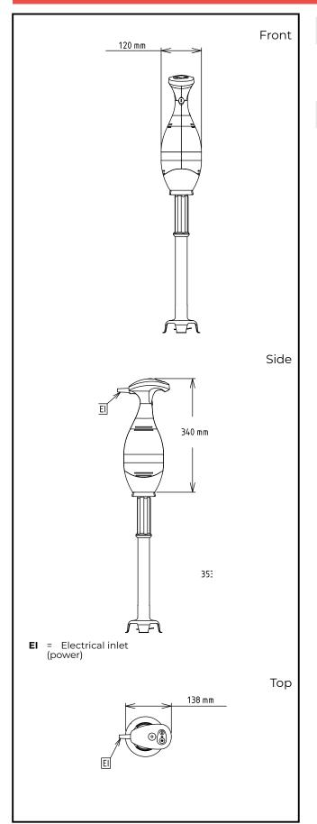
Electric Supply voltage: 600309 (DBPU350) 220-240 V/1 ph/50/60 Hz Electrical power max.: 0.35 kW **Total Watts:** 0.35 kW Key Information: External dimensions, Width: 138 mm External dimensions, 120 mm Depth: External dimensions, Height: 340 mm **Shipping weight:** 3 kg
